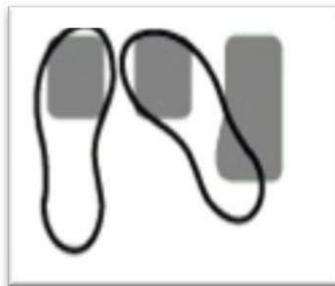
Fig.1: Schematic representation of operating the brake, clutch and accelerator simultaneously
