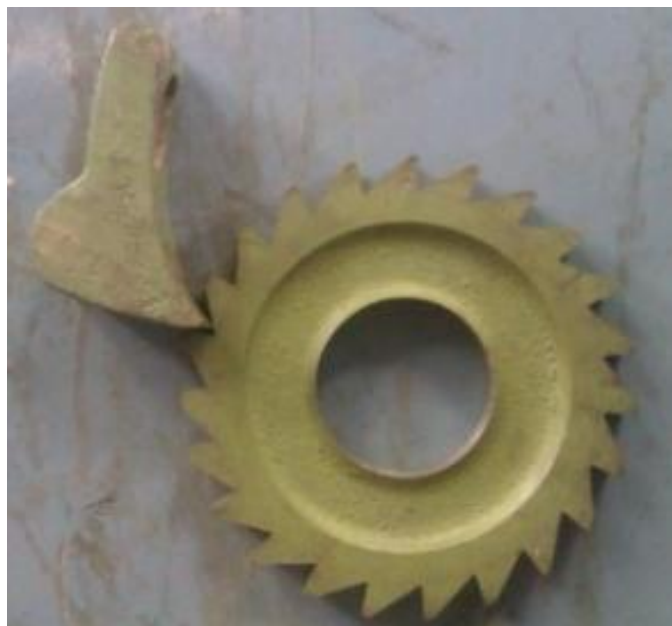
Fig. 3: Fabricated Ratchet and Pawl mechanism
